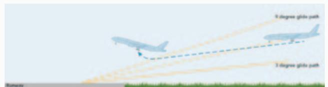
Figure 2: Example of glide slope capture with a pitch upset above 3 degree glide path.
